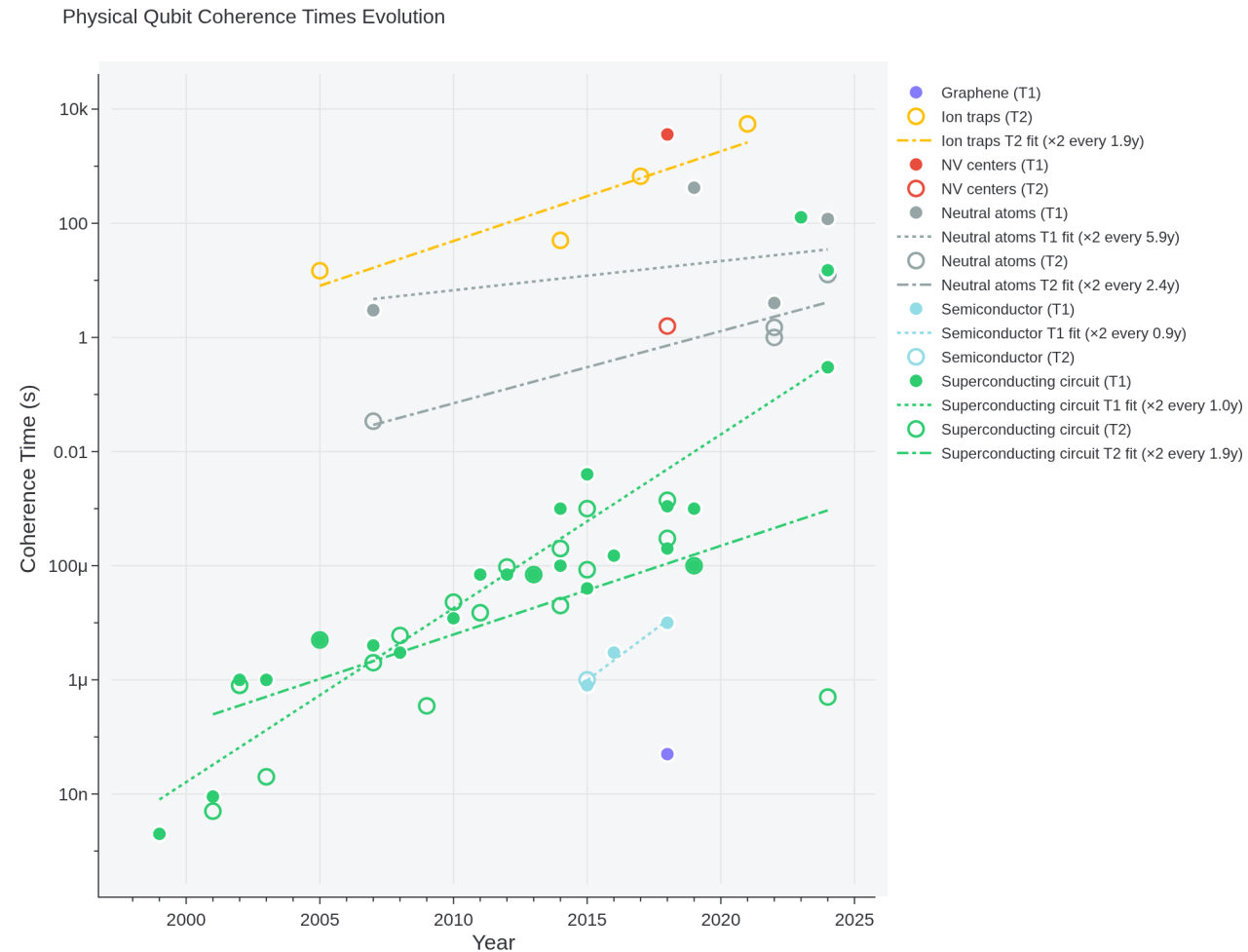
Figure 7: Evolution of T_1 and T_2 times over two decades. See Awesome Quantum Computing Experiments .
