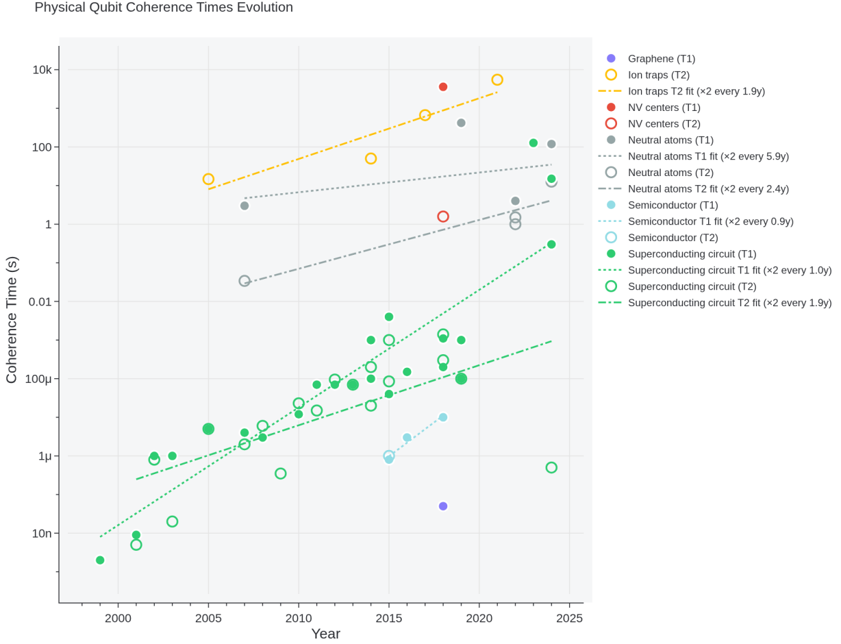
Figure 8: Physical qubit bitflip and coherence times. Evolution of reported T_1 in solid lines and T_2 in dashed lines, times across different platforms. An exponential fit showing the characteristic doubling time in years is included. For superconducting circuit, the T_1 \times 2 every 0.99y, and for T_2 every 1.94y.
