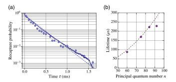
FIG. 4. (a) Recapture probability of a  $84S_{1/2}$  Rydberg atom, as a function of the time spent in the BOB trap, showing a roughly exponential decay with lifetime  $222 \pm 3 \mu s$  (dashed line). The solid line is the result of a simulation without any adjustable parameter (see text). (b) Measured lifetimes of various  $nS_{1/2}$  states; the dashed line is the theoretical value [46].
