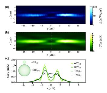
FIG. 2. (a) Example of measured light intensity distribution near the focal plane. (b) Trapping potential for the  $84S_{1/2}$  Rydberg state calculated from Eq. (1) and the intensity distribution shown in (a). (c) Cuts of the trapping potential along z=0 [dashed line in (b)] for different  $nS_{1/2}$  Rydberg states. Schematics of the 60S and 120S Rydberg orbitals (to scale) are shown as insets.
